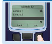
Highlight the ID and select 'OK'. The screen shows the option to select either 'Edit' to change the ID, or 'Delete'. Deleting the sample ID will not affect results stored in the log.
