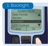
The instrument display features a high intensity backlight for use in low light conditions. Select either 'On' or 'Off'.
