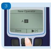
Use the Up/Down buttons to select characters. When the correct character is shown, press and hold the [+] key to move to the next character. To delete characters press and hold the [Del] key. Select 'Done' to save the ID.
