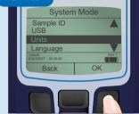
To change units which results are shown in, from the home screen press 'System' mode then 'Units'.
