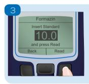
The instrument will request the remaining standards in order of increasing turbidity value. After the final standard has been read, the screen will show a countdown timer. When the calibration process is complete the screen will show 'Successful'.
