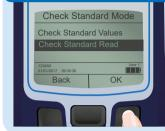
Select the Check Standard Read option to perform a recorded reading of each turbidity check standard.
