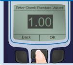
Use the up/down keys to adjust the displayed values to match the assigned target for each check standard.
