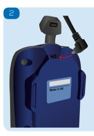
Once the device is in 'Hard Drive' mode connect to a PC, using the supplied USB cable. З
