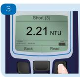
An audible tone will sound at the start and end of measurement. Result is displayed on the screen and stored in the log with time, date, Reading Mode, Operator ID and Sample ID.
