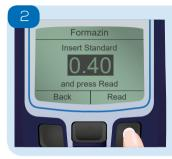
Insert the lowest turbidity value calibration standard when prompted. Use the Up/Down buttons to adjust the value on screen to that on the standard and press 'Read.
