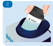
Insert the sample with the orientation mark ◊ facing forward and press 'Read'. An audible tone will sound at the start and end of measurement.
