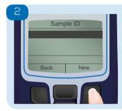
To create a new Sample ID Scroll to the bottom of the list, then select 'New'. Use the Up/Down buttons to select characters. When the correct character is shown, press and hold the [+] key to move to the next character.
