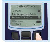
Select 'Calibrate/Check' from the main menu then 'Restore Factory Calibration'. Select 'YES' to confirm the restoration.
