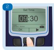
Use up/down keys to adjust the hour; press the right key to select and adjust the minutes. The time is displayed in 24Hr format.
