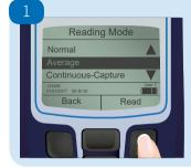
This mode takes multiple measurements and averages the results. Three options are available: Short (3 readings), Medium (6 readings) and Long (12 readings).
