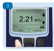
Results are not stored automatically. To store a result in the log, press 'Capture' (repeat as required). To stop measurement, press 'Stop' at any time.
