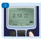
'Pass' will appear onscreen if the result is within the tolerance displayed on the standard. If the result is outside of the tolerance, the instrument may need to be re-calibrated.
