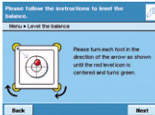
Q-Level combines novel sensors with the most advanced display technology, making it easier and faster to level the balance accurately. A standard feature of Cubis MSA and MSU display and control units, interactive prompting guides you during manual leveling. The display provides all the necessary information: the position of the air bubble and instructions regarding which leveling foot
