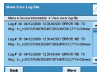
The audit trail function logs major changes to the device. In this way, errors can be tracked quickly.
