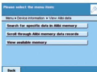
An integrated Alibi memory for traceable transfer of legal-fortrade weighing data to a PC.
