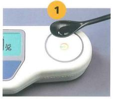
Apply drops of sample into the sensor section until it fills above the indication line.
